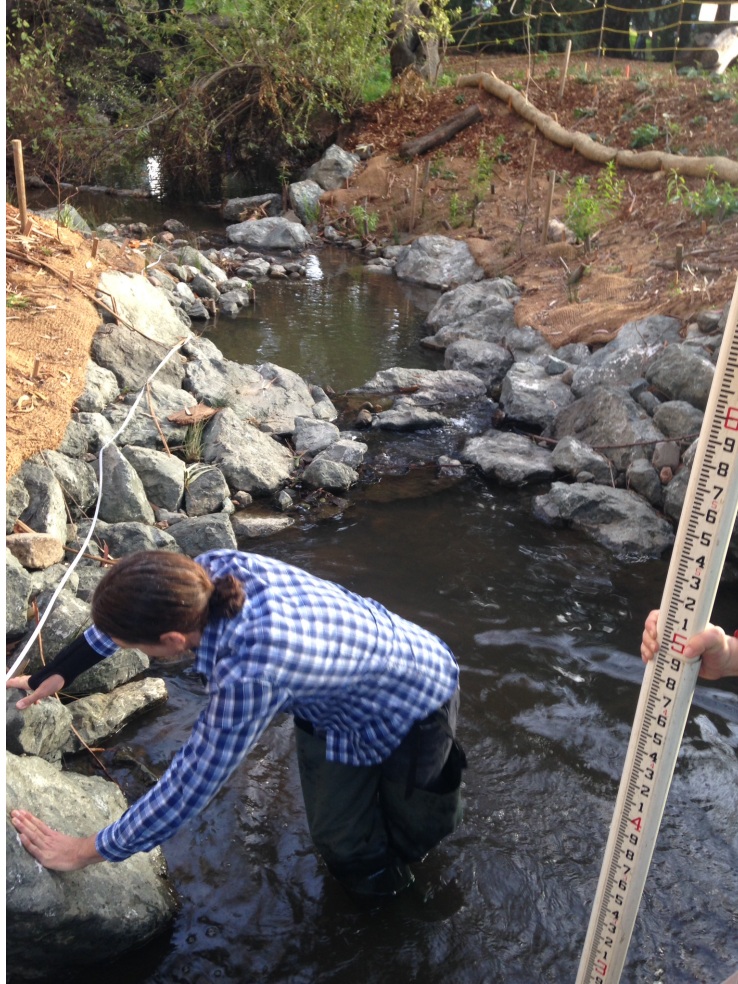
Figure 8. The long profile was surveyed by running the measuring tape along the left stream bank to mark the station while using the survey stick to locate the deepest portion in the creek. Relative elevations were recorded through viewing the numbers on the meter stick through a survey tool which was stationed in a spot without any large obstructions. If we had continued to survey further along the stream, we would have needed to take a turning point elevation measurement to relocate the survey tool to keep the measuring stick within view.
