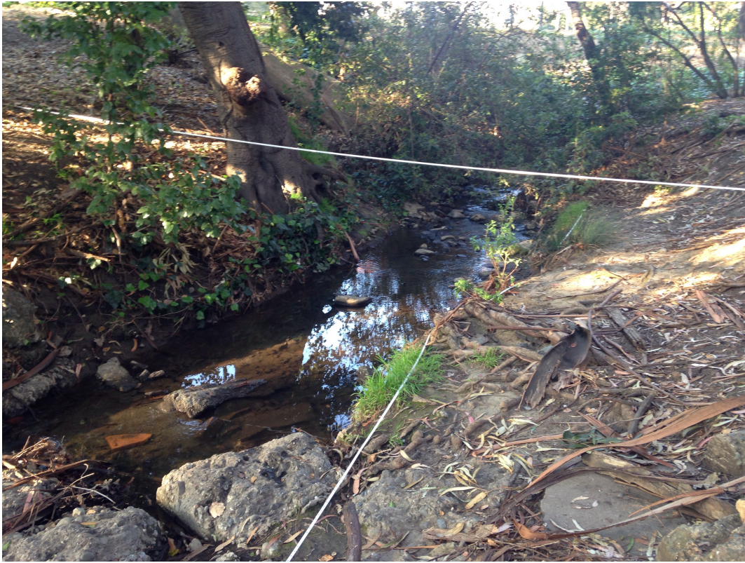
Figure 6. The measuring tape across the stream marks the non-restored cross-section that was surveyed (upstream-facing). The sandy area on the left bank reveals a potential high water mark from a recent flooding event.
